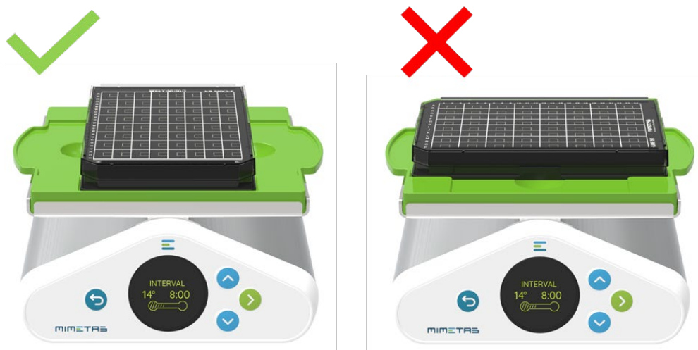
Figure 7: Place the OrganoPlate® on the OrganoFlow® in the correct orientation.
